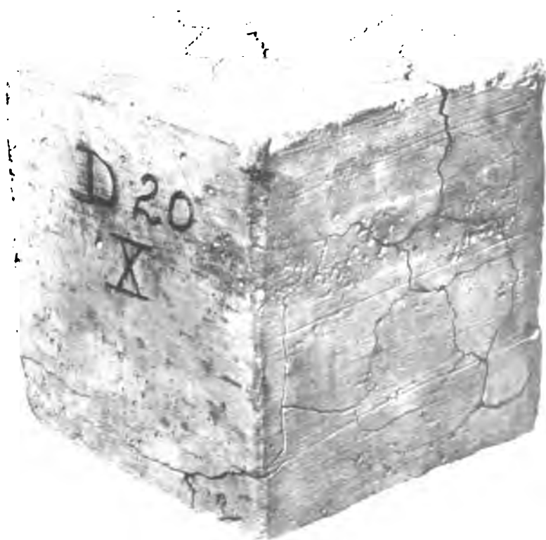
4 INCH CUBE D20, DYCKERHOFF CEMENT. APPEARANCE 6 DAYS AFTER HAVING BEEN HEATED TO 100° C. (212° F.)
